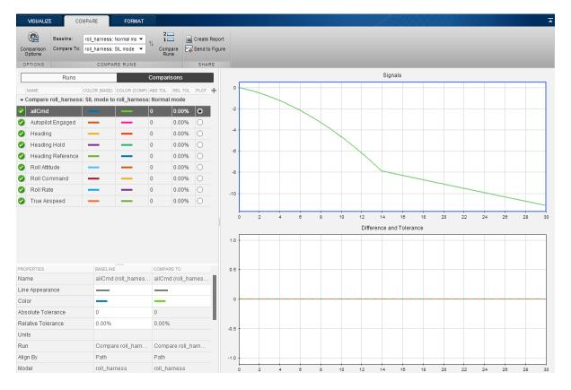
If you find differences in testing results, it is important to investigate and understand the differences. Some differences can be attributed to implementation changes (converting from an interpreted model to an executable implementation), or can be an indication of bugs. You must understand all differences to confirm that the behavior of the system is free of bugs.
